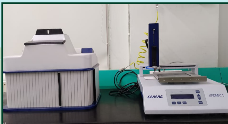
High performance Thin Layer Chromatography (Make - CAMAG Linomat 5)
