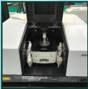
Fourier Transform Infrared Spectrophotometer (FTIR) (Make- Shimadzu)
