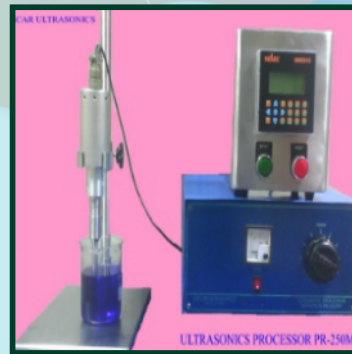
Probe Sonicator (Make: Oscar Ultrasonic)
