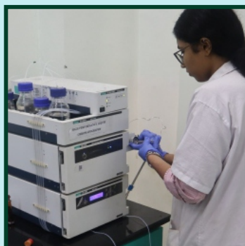
High Performance Liquid Chromatography with PDA (Make- Jasco)
